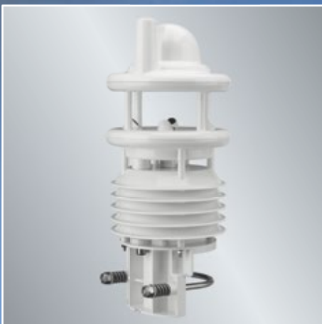
The wind sensor is heated and has no mechanical moving parts (static wind sensor). The sensor measures 16 times per second. The quality value in the measurement output shows the number of valid measurements that are within the permitted measurement interval.
