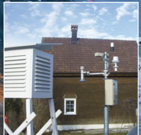
Today, meteorological systems use both, a present weather sensor and a precipitation gauge. In future, the WS100 can replace both sensors.
