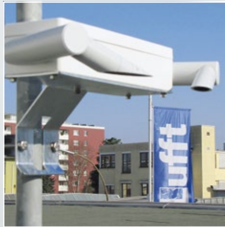
Verification in the field is carried out using a calibration disc. As a further control point, the zero point is checked ("in the dark").
