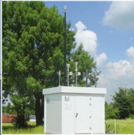
WS600: Radar technology is used for maintenance-free recording of precipitation. WS700 measures irradiance in addition.
