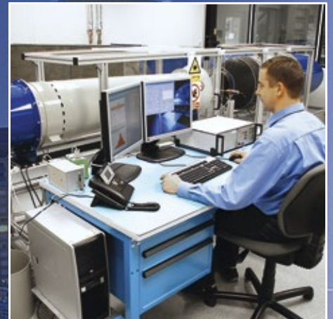
In the field, typically only two measuring points can be verified: calm and the current wind speed. In the laboratory, the sensor is calibrated and adjusted over the entire relevant measuring range. The measurement certificate for each sensor provides information about the actual accuracy, which is generally significantly better than the technically specified minimum accuracy.
