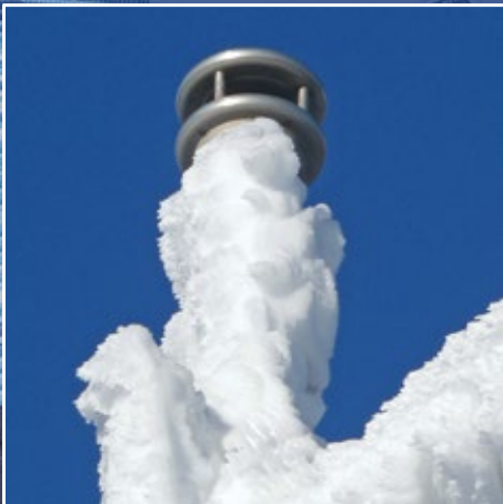
Ice usually forms first on the measuring mast. In critical applications, therefore, the mast mount is heated. The wind sensor is heated on the upper and lower plates. In the X-version, the measuring heads are also directly heated.
