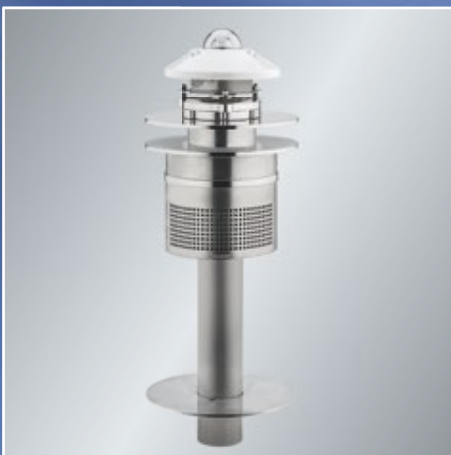
Optional: WS3100 with pyranometer (secondary standard).
