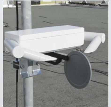
The degree of contamination of the sensor is transmitted together with the measured values and serves to alert proactive maintenance.
