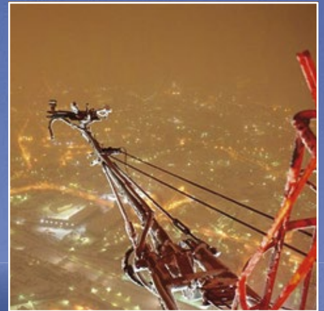
Ice-free test in Ostankino, Moscow. The television tower is 600 m high and in the winter often stands in an ice cloud.
