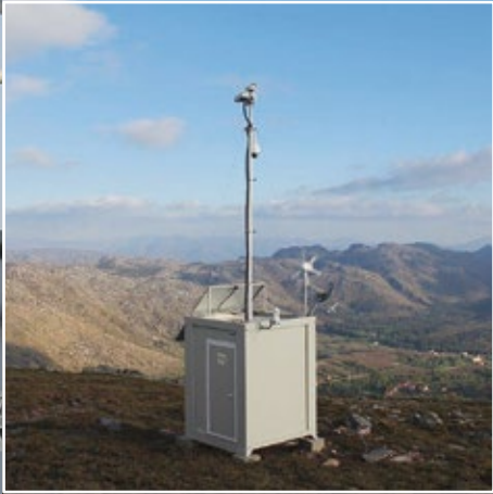
For meteorological applications the WS 500 is combined with a tipping bucket for precipitation measurement.
