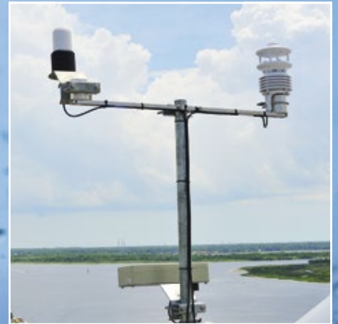
All UMB-sensors use the same output protocol. This allows easy integration into any new or existing system design.
